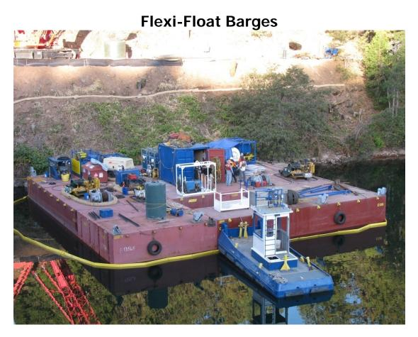
The 20' x 10' or 40' x 10' barge sections are transported to the site on tractor-trailers, then assembled in the water.
